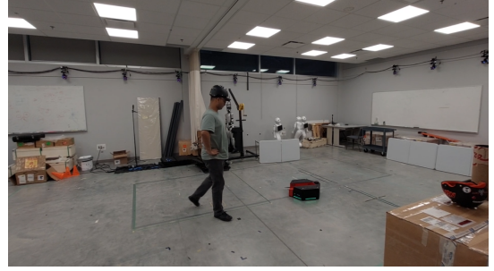
Fig. 1. Real-world deployment of the MCTS-DRL follow-ahead system on a QBot robot tracking a person.
